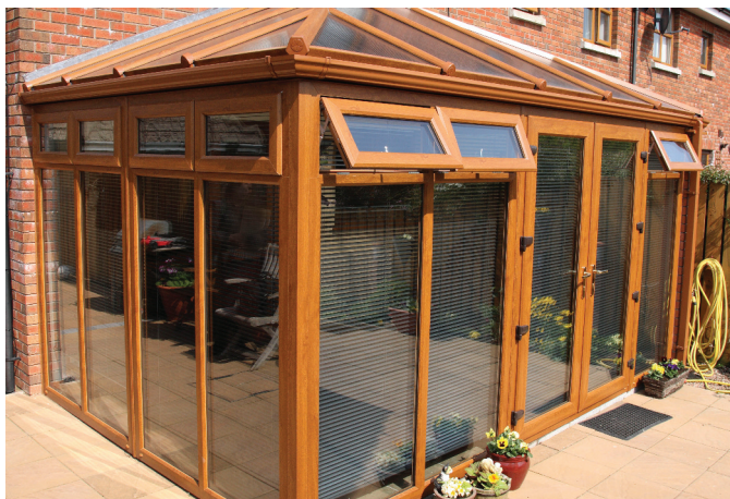
Light Oak Single Edwardian with frames to floor (and 35mm bronze polycarbonate in roof). Note: No sill to bottom of frames, frames overhang threshold by 5-7mm to create drip & cleaner lines.
